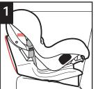
Place child restraint rearfacing in the back seat. With child restraint in the fully reclined position, make sure level line on side of shell is level with
